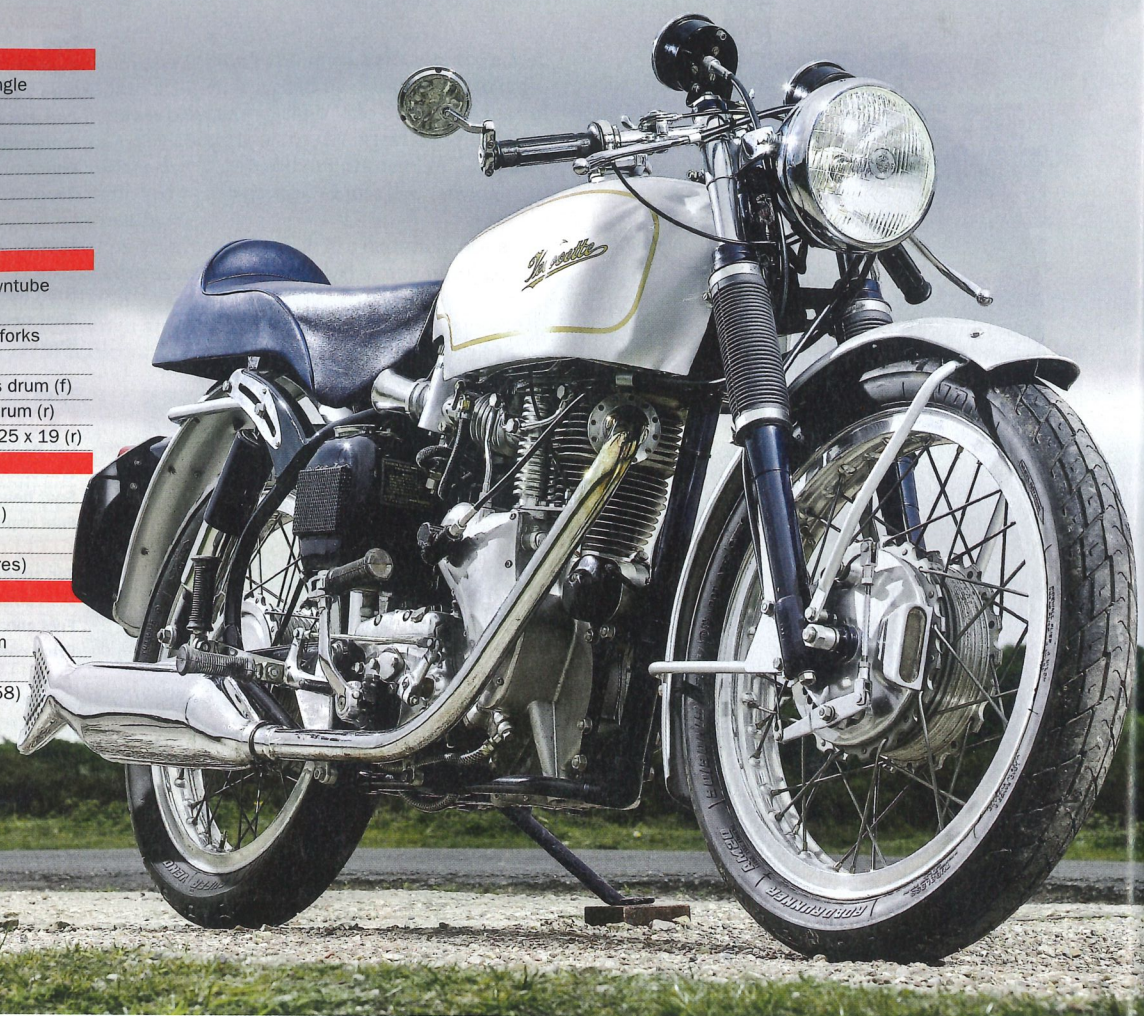
■ Cut-out in tank accommodates the Amal Monobloc
