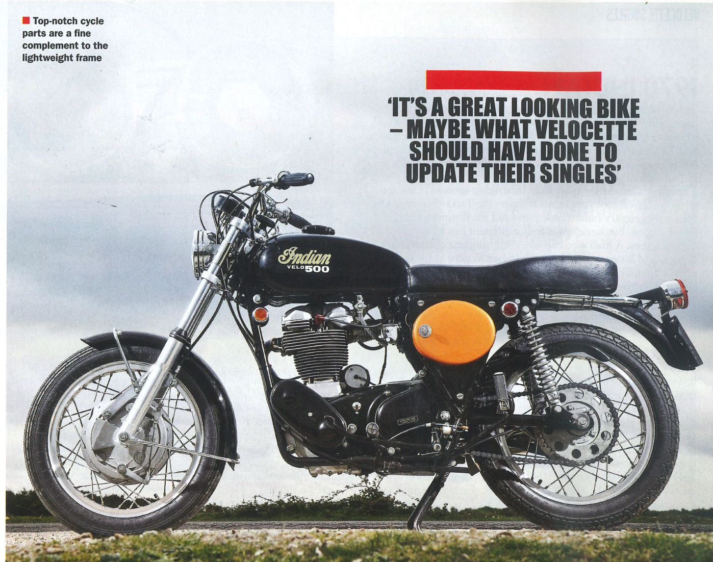
■ Thruxton engine mated to Tartarini frame made Clymer's dream, but buyers didn't agree
