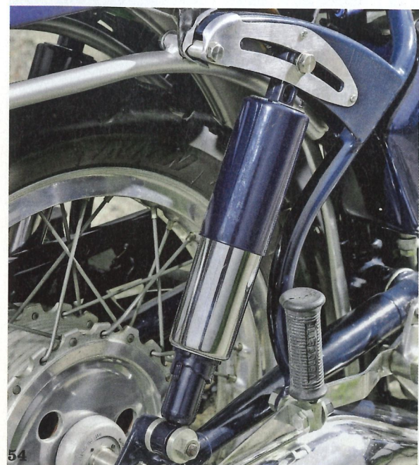
■ Below: Adjustable shock absorber mounts are another Velo hallmark
